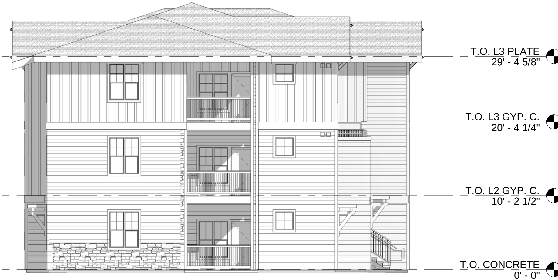
3 BUILDING B - LEFT ELEVATION 1/8" = 1'-0"
