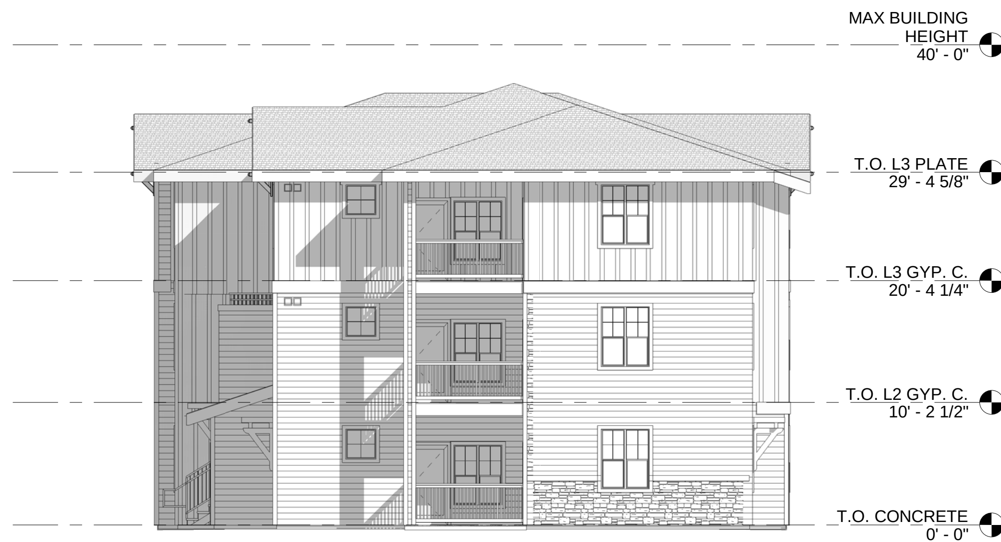
2 BUILDING B - RIGHT ELEVATION 1/8" = 1'-0"
