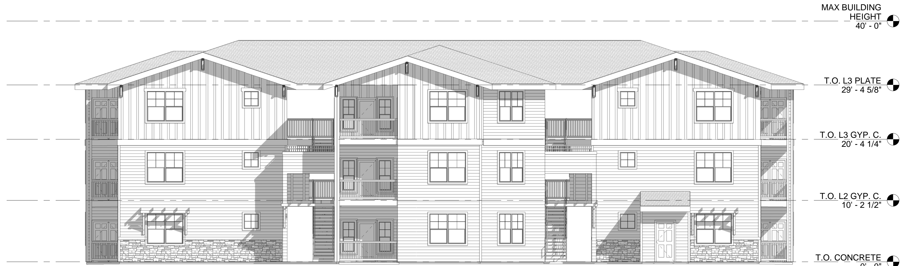
1 BUILDING B - FRONT ELEVATION 1/8" = 1'-0"
