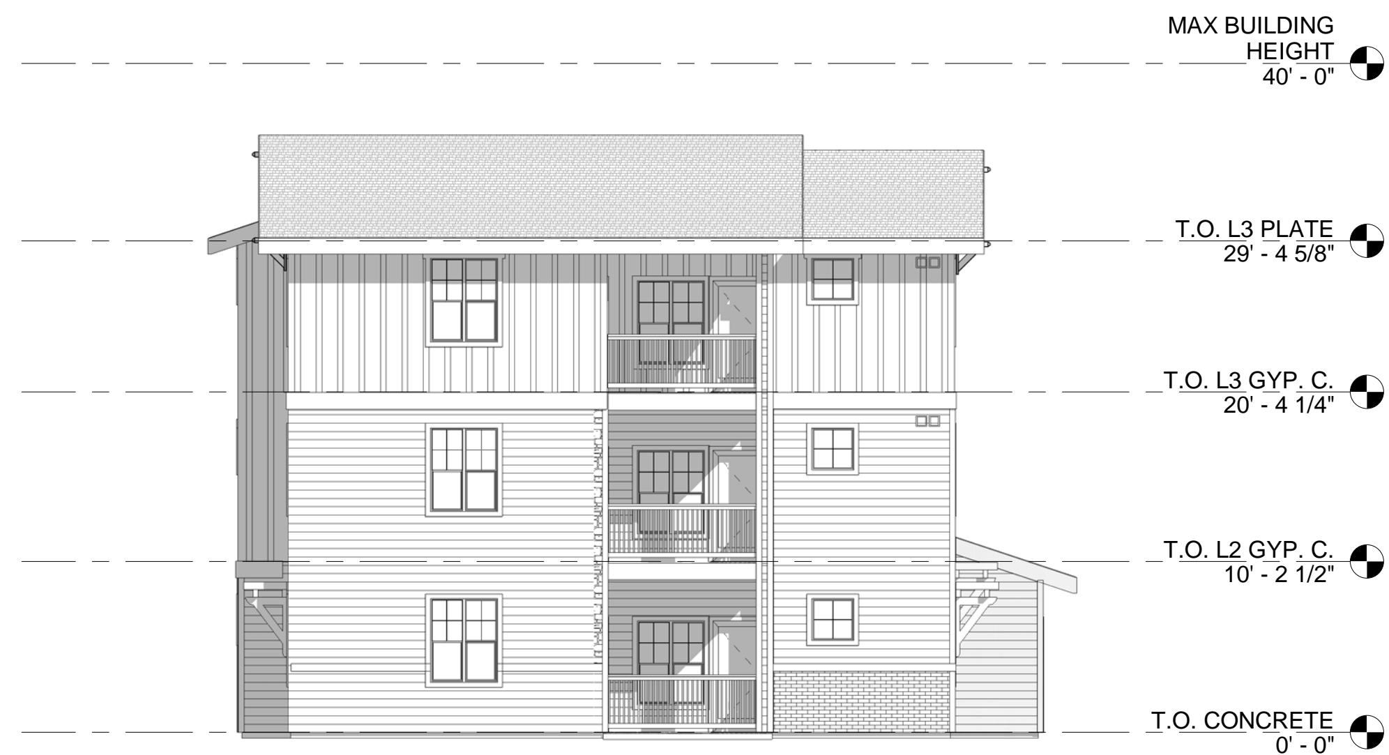
5 BUILDING C - LEFT ELEVATION 1/8" = 1'-0"
