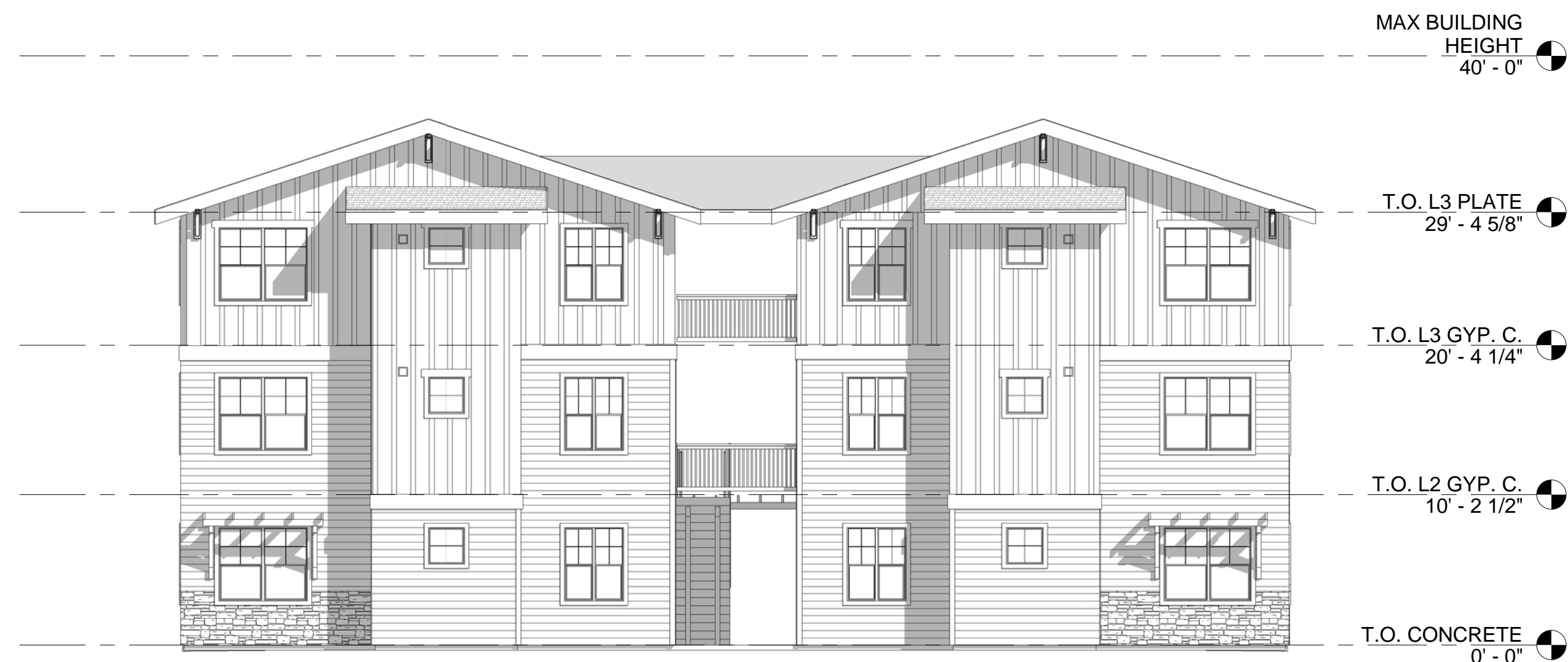
3 BUILDING C - REAR ELEVATION 1/8" = 1'-0"
