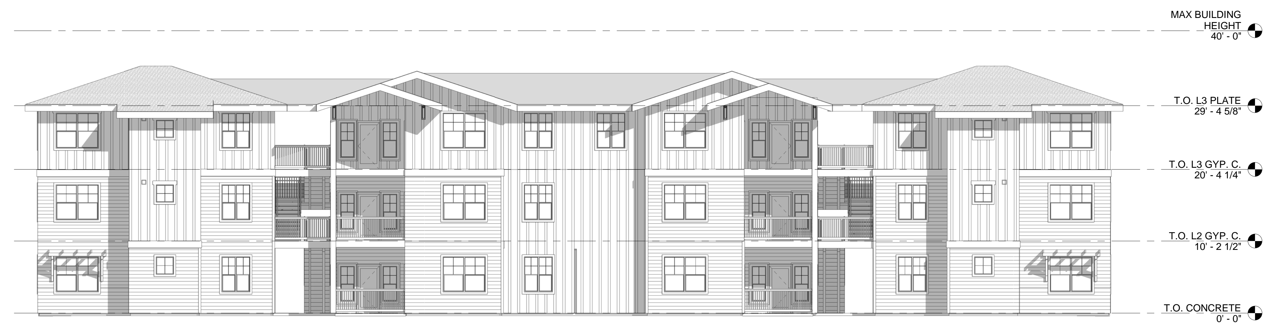
3 BUILDING A - REAR ELEVATION 1/8" = 1'-0"
