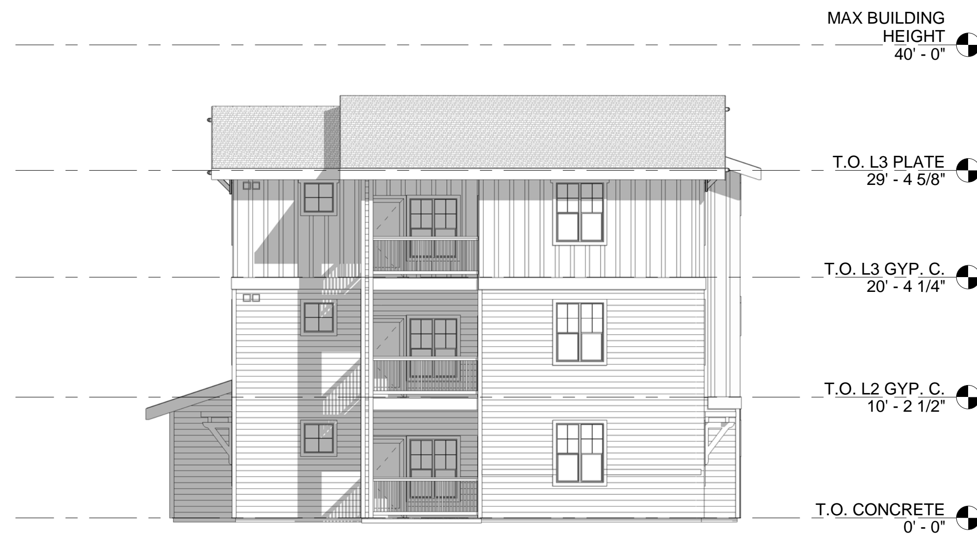
4 BUILDING C - RIGHT ELEVATION 1/8" = 1'-0"
