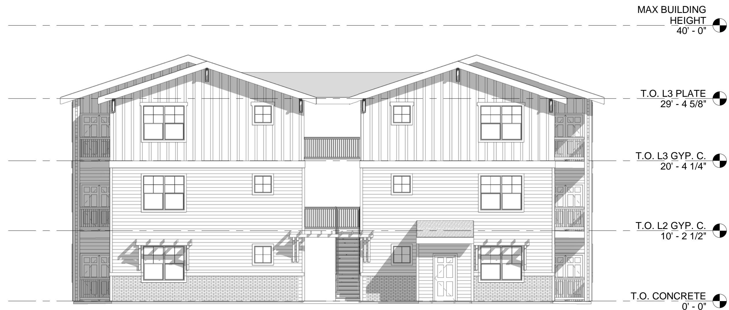
1 BUILDING C - FRONT ELEVATION 1/8" = 1'-0"
