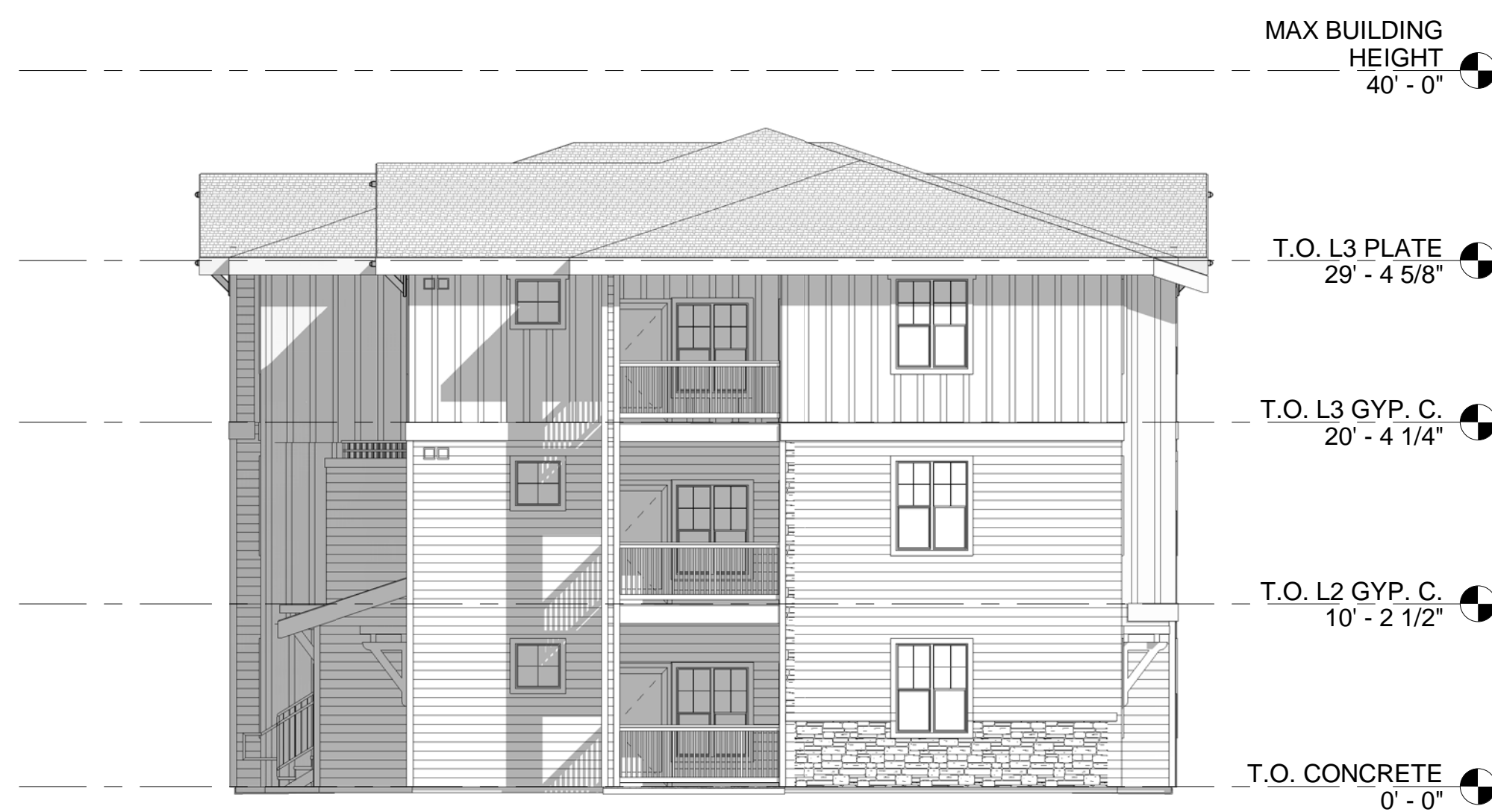
2 BUILDING B - RIGHT ELEVATION 1/8" = 1'-0"
