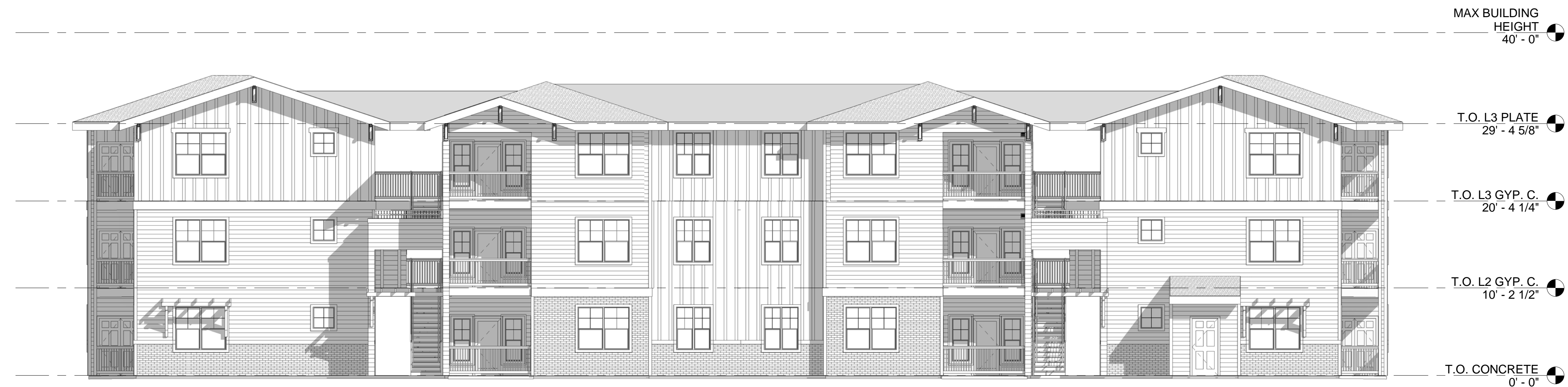
1 BUILDING A - FRONT ELEVATION 1/8" = 1'-0"
