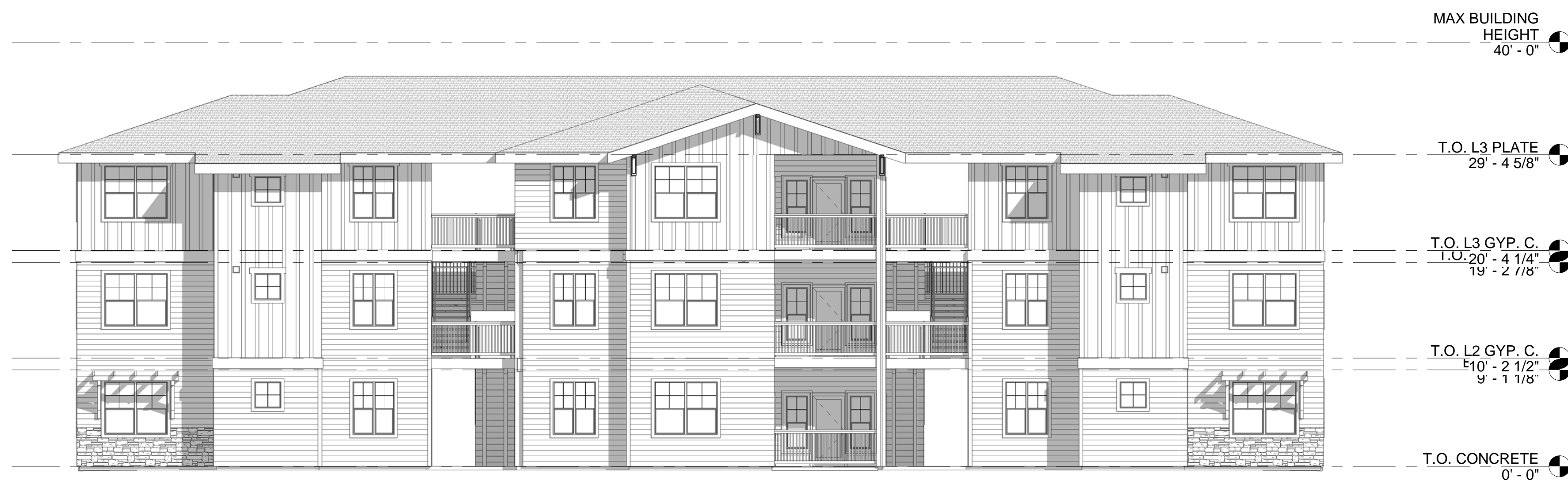
4 BUILDING B - REAR ELEVATION 1/8" = 1'-0"
