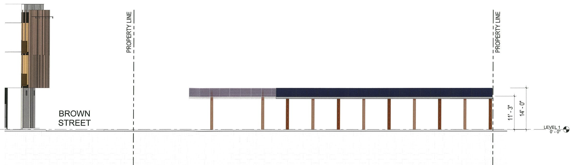
2 SOLAR CARPORT ELEVATION - DEPOT 1/8" = 1'-0"
