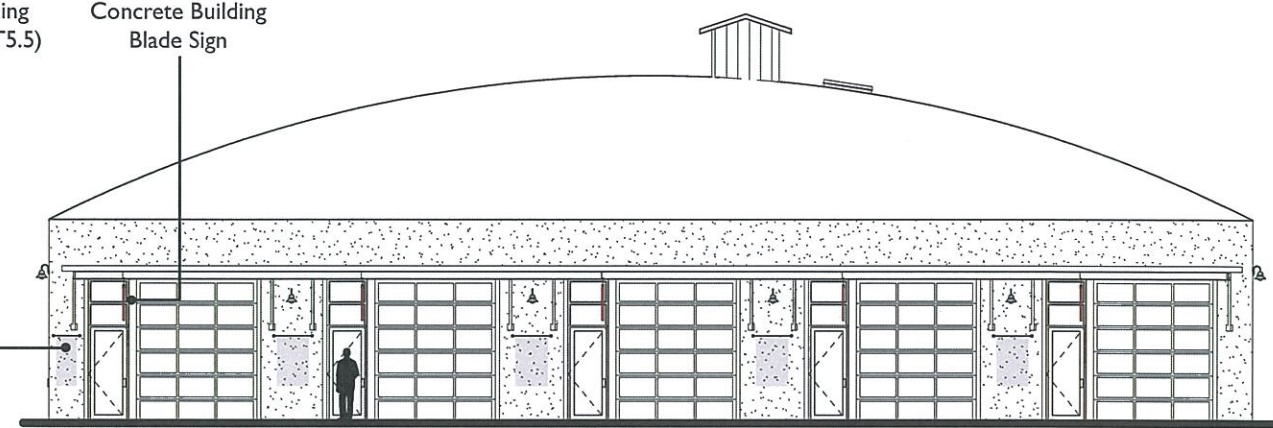
6780 CONCRETE BUILDING SOUTH ELEVATION Scale: 1/16" = 1'-0"
