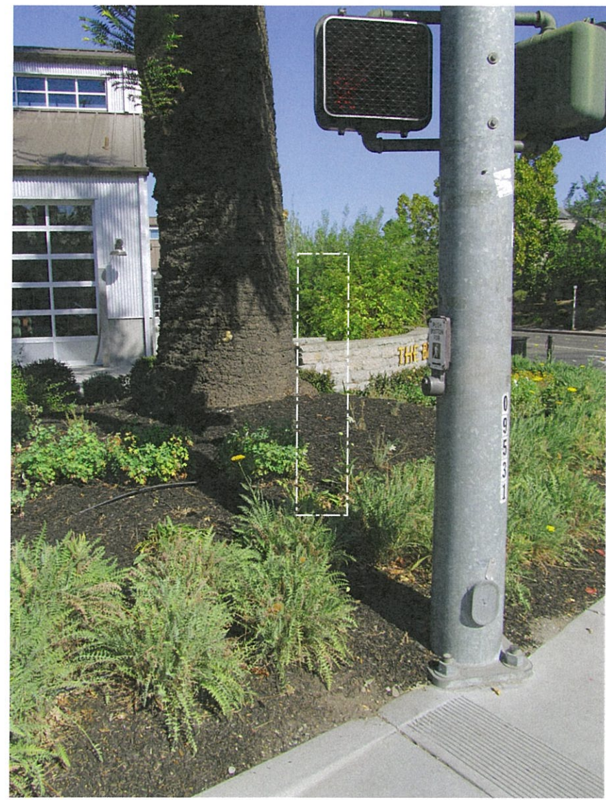
Center B1 sign between tree and traffic light but staying with 5' min from property line.
