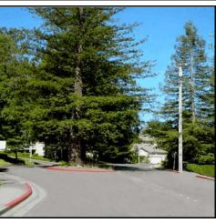
**Bulbouts** were used as part of a new residential subdivision on Robinson Road, which is mix of narrow rural street sections with pockets where the street is widened and has curb, gutter and sidewalk. The intent of the bulbouts, which are maintained by the subdivision, is to "shadow" the onstreet parking, which is generally not used, and to provide a transition between the unimproved narrow section and the pockets of widening.
