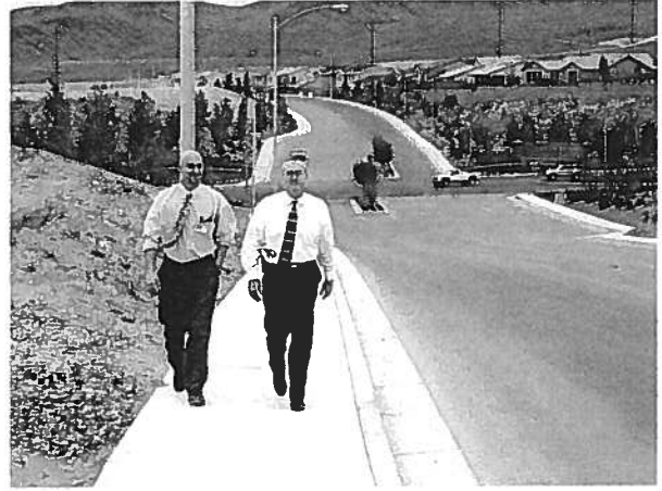
Our desire to walk or avoid a walk is based on quality of experience. Attached sidewalks require a buffer. Planter strips of 6-7 feet are ideal. On street parking and bike lanes offer buffers when the sidewalk must be attached to the curb.
