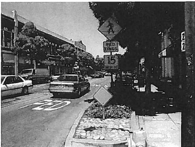
There are several sites on Main Street where bulb outs can be placed to improve pedestrian crosswalks without losing parking. Bulb outs help make pedestrians more visible to motorists and add space for landscaping.
