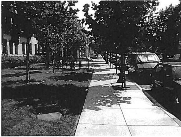
Citizens want more trees. Tree wells and trees in adjacent landscaped areas allow the trees to canopy over the walkway. Tree wells can also be placed between every two to four parked cars with no significant loss of parking spaces.
